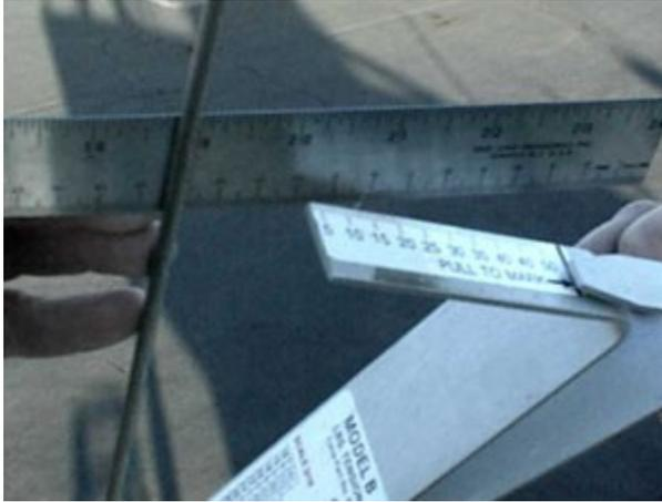
4) Now tighten the upper shrouds to 24 on a Loos Model B tension gauge ([See Tension Gauge Conversion Chart](#)) and the lowers to 21. We get the uppers snug first and then using the genoa halyard measure down to the chainplates on both sides to be sure the mast is centered in the boat. Be sure to sight up the backside of the mast to be sure it is straight.
