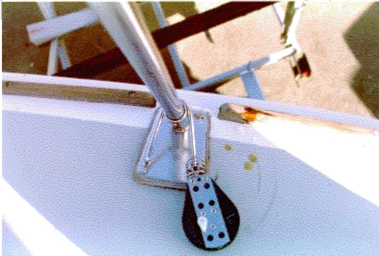
Stanchions and bases are particularly susceptible to damage. Notice the cracks that run under the base of this stanchion - a good clue that there may be some damage. But notice how carefully the holes from old hardware have been filled.
